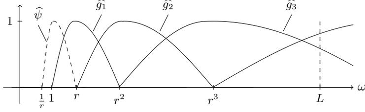
Figure 3: Illustration of the Fourier transforms of the wavelet filters  $g_j$  on the frequency band  $[0, L]$ . The Fourier transform  $\widehat{\psi}$  of the mother wavelet  $\psi$  is supported on the interval  $[r^{-1}, r]$ .
