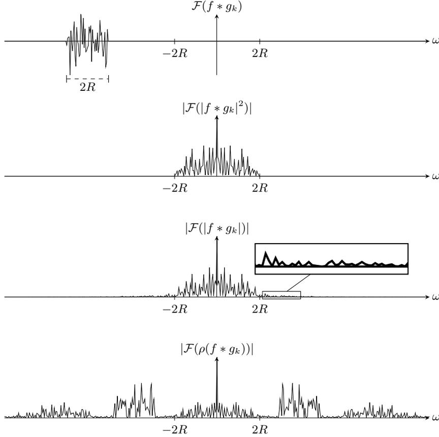
Figure 6: Illustration of the demodulation and bandwidth doubling effect of the squared modulus (second row) and the modulus non-linearities (third row). The WH filters have prototype function  $g$  with  $\text{supp}(\hat{g}) = [-R, R]$ . The rectified linear unit non-linearity (bottom row) is defined as  $\rho(z) := \max\{0, \text{Re}(z)\} + \max\{0, \text{Im}(z)\}$ ,  $z \in \mathbb{C}$ .
