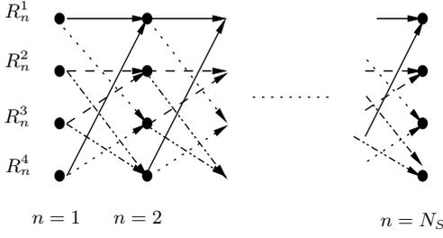
FIGURE 3 - TRELLIS USED IN THE MLSD OF DBP CODES.
