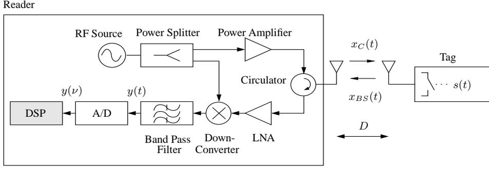
FIGURE 1 - RFID SYSTEM USING BACKSCATTERING MODULATION.
