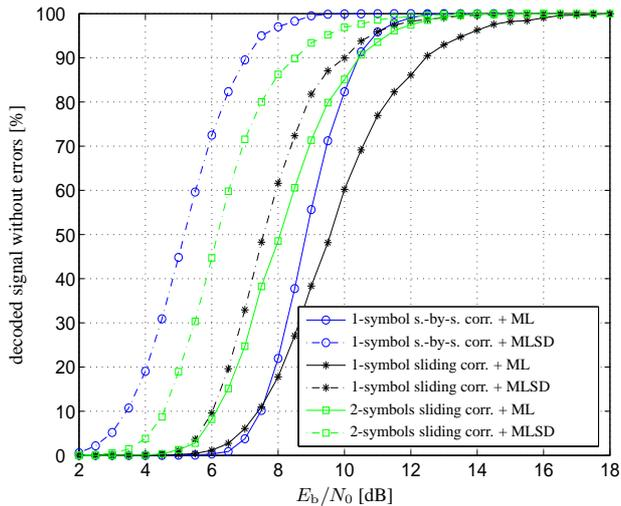
FIGURE 5 - PERCENTAGE OF DECODED DATA SIGNALS WITHOUT ERRORS APPLYING SYMBOL-BY-SYMBOL AND SLIDING DETECTIONS.
