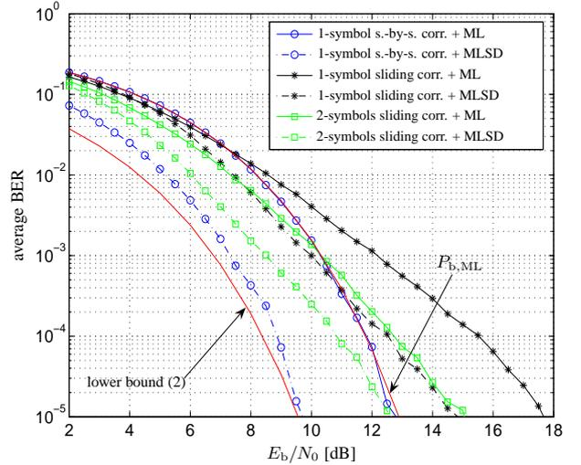
FIGURE 4 - AVERAGE BERs APPLYING SYMBOL-BY-SYMBOL AND SLIDING DETECTIONS.
