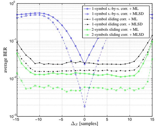
FIGURE 6 - AVERAGE BERS AT 7 dB APPLYING SYMBOL-BY-SYMBOL AND SLIDING DETECTIONS AS A FUNCTION OF THE TIME SAMPLE ERRORS.
