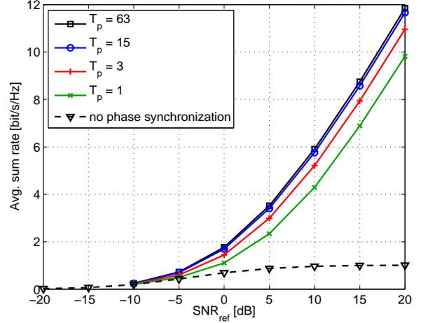
Fig. 5. Average sum rate vs.  $\text{SNR}_{\text{ref}}$  assuming absence of phase noise
