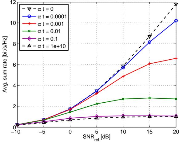
Fig. 4. Average sum rate vs.  $\text{SNR}_{\text{ref}}$  assuming absence of additive noise
