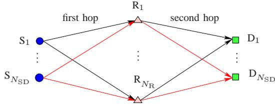
Fig. 1. System configuration for a two-hop relay network
