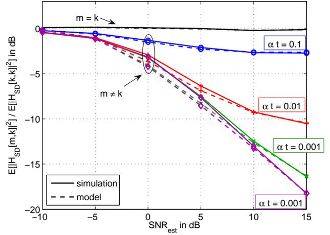
Fig. 3. Normalized expected power of the equivalent channel
