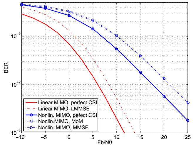
Fig. 6. BER of a  $2 \times 2$  MIMO system.  $N_{\text{tot}} = 3$ .
