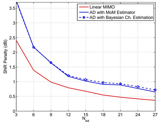
Fig. 7.  $2 \times 2$  system,  $\text{BER}=10^{-2}$ . SNR penalty of various estimation methods with respect to perfect CSI, as a function of  $N_{\text{tot}} = 3N$ .
