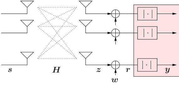
Fig. 1. MIMO System Reference Model
