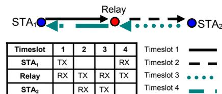
Fig. 1 Conventional DF relaying using half-duplex relays
