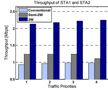
Fig. 3 Throughput of conventional, semi-2W and 2W relaying
