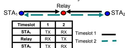
Fig. 2 Two-way DF relaying using half-duplex relays
