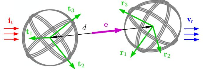
Fig. 2. Magneto-inductive  $3 \times 3$  MIMO link between collocated, orthogonal coil arrays. TX current vector  $\mathbf{i}$  induces voltage vector  $\mathbf{v}_r = j\omega \mathbf{M} \mathbf{i}_t$  at the RX array.  $d$  and  $\mathbf{e}$  are analogous to the  $1 \times 1$  case due to collocation.
