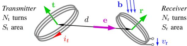
Fig. 1. Magneto-inductive  $1 \times 1$  link between single coils with separation  $d$ . TX current  $i_t$  induces voltage  $v_r = j\omega M i_t$  at the RX coil. Unit vector  $\mathbf{e}$  points from TX to RX, while unit vectors  $\mathbf{t}$  and  $\mathbf{r}$  describe TX and RX coil orientations, respectively.
