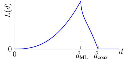
Fig. 6. Ranging likelihood function  $L(d) = f_{M|d}(M_{\text{meas}}|d)$  for a mutual inductance measurement  $M_{\text{meas}}$  (assumed noiseless).  $\hat{d}_{\text{ML}}$  is the maximum likelihood range estimate.
