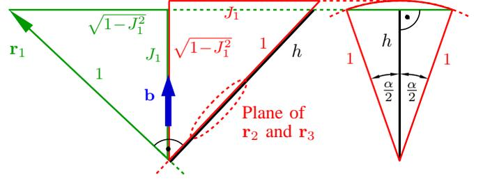
Fig. 3. Sketch of the transitional case in single-sided coil selection. Shown are the front view on the left-hand side and a lateral view to the right-hand side. For  $\frac{1}{\sqrt{3}} < |\mathbf{r}_1^T \mathbf{b}| / \|\mathbf{b}\| < \frac{1}{\sqrt{2}}$ , the coil with orientation  $\mathbf{r}_1$  may or may not have strongest coupling, depending on orientations  $\mathbf{r}_2$  and  $\mathbf{r}_3$ .
