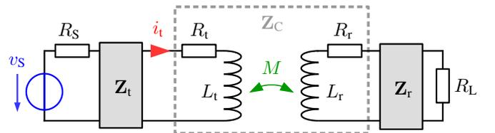
Fig. 7. General circuit model of a magneto-inductive  $1 \times 1$  link.
