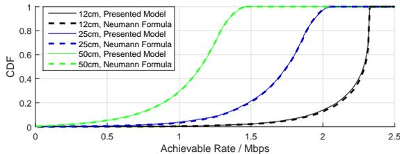
Fig. 8. Model comparison in terms of rate CDFs at different separations. Flat circular coils of 5 cm diameter were assumed. Reference values were computed with the Neumann double line integral. Parameter  $N_t = N_r = 5$ ,  $f_c = 25.4$  MHz,  $B = 100$  kHz,  $P_{\text{TX}} = 1$   $\mu$ W, LNA noise figure = 15 dB.
