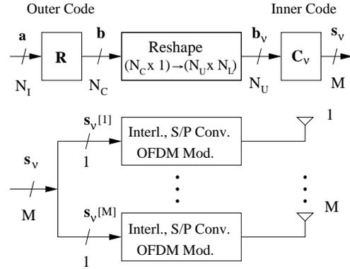
Fig. 2. Symbol discrete model of the LSD encoding scheme
