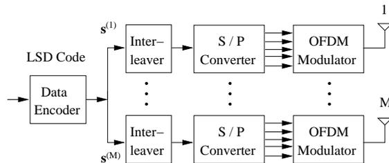
Fig. 1. System block diagram of a space-frequency coded OFDM transmitter
