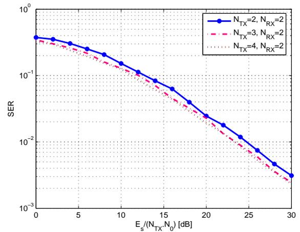
Fig. 4. Symbol error rate for MIMO systems using antenna selection combining
