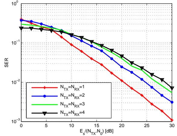
Fig. 3. Symbol error rate for MIMO systems using time domain precoding with power constraint at the transmitter for a 3-taps channel with uniform power delay profile
