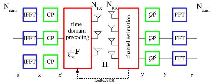
Fig. 1. System model. The noise source has been omitted
