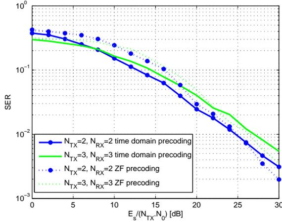
Fig. 2. Symbol error rate for time domain precoding and frequency domain zero forcing precoder for a 3-taps channel with uniform power delay profile
