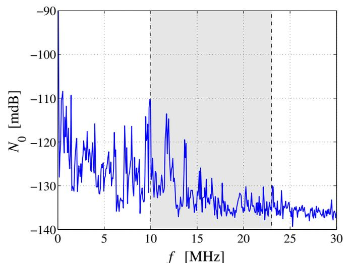
Fig. 5. Measured power density spectrum for the average channel
