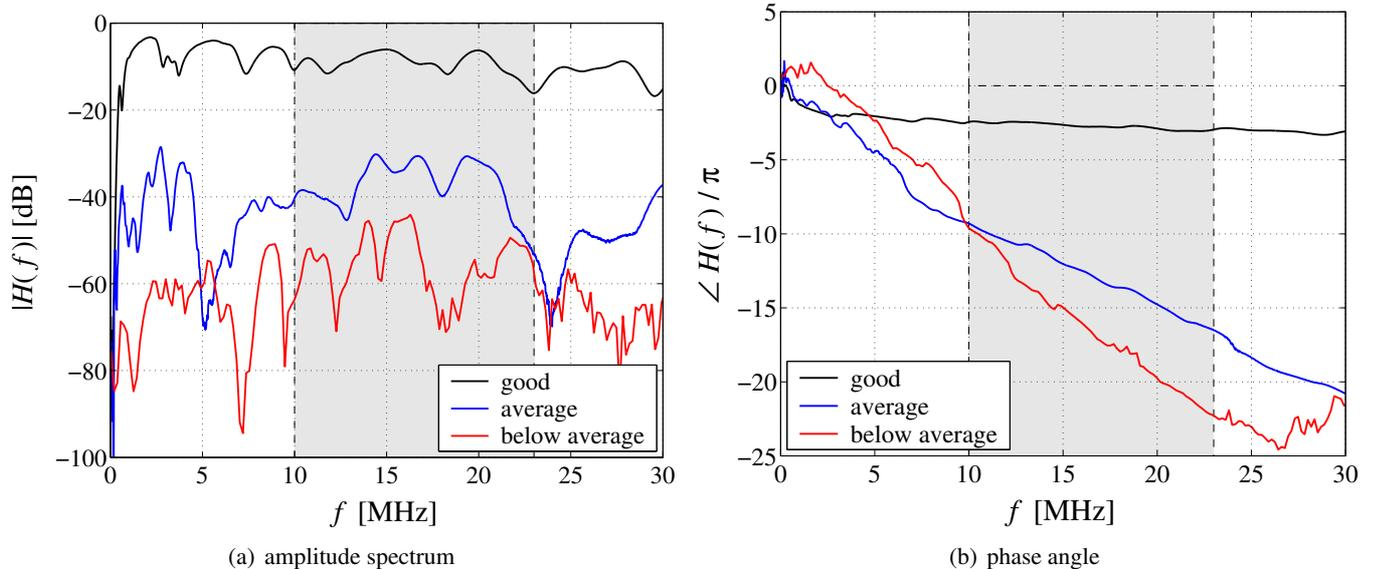
Fig. 4. Three measured PLC transfer function
