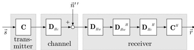
Fig. 2. System model for the linear block code and the OFDM
