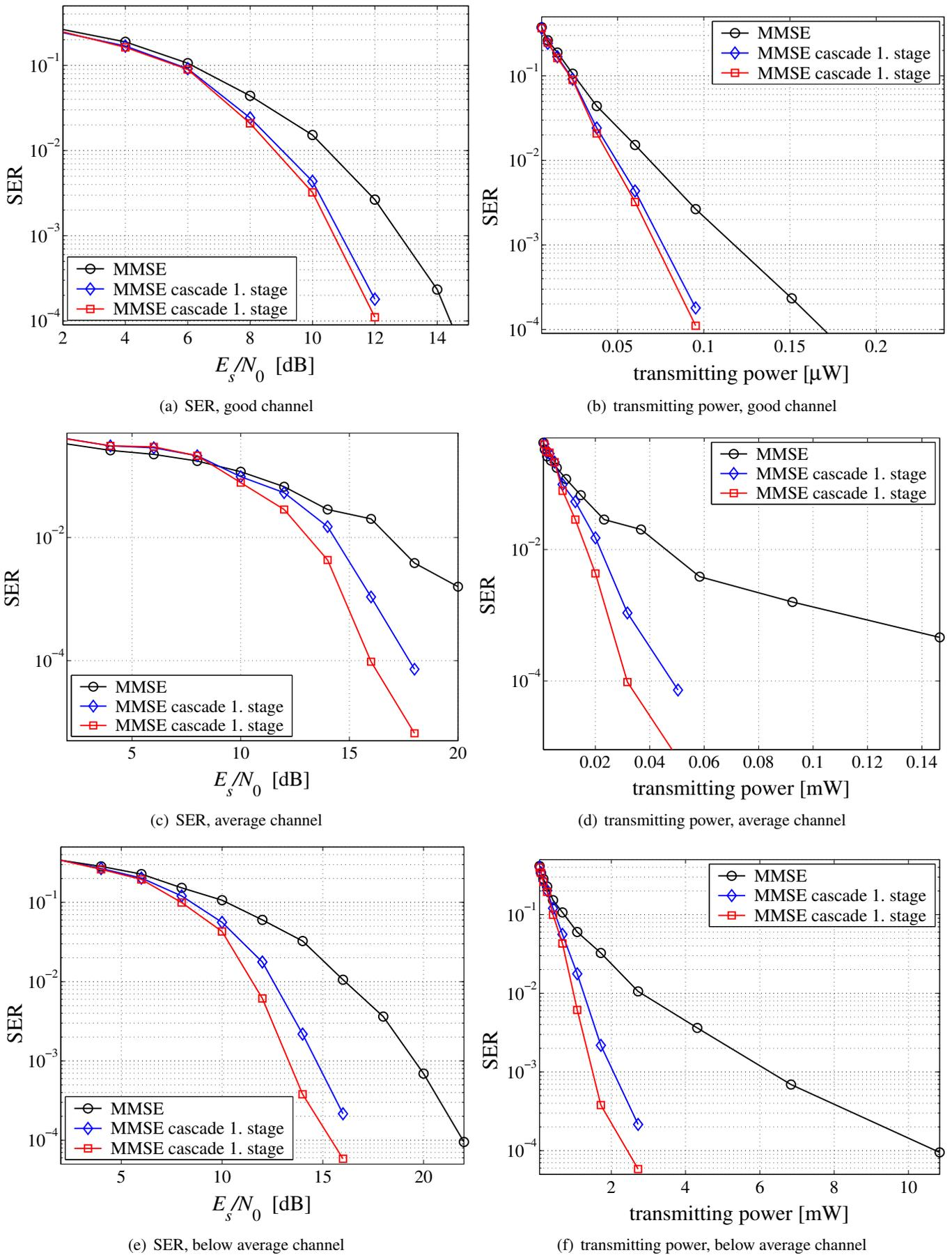
Fig. 6. SER versus  $E_s/N_0$  and versus the transmitting power for the three measured transfer functions
