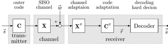
Fig. 1. System model for the SISO channel
