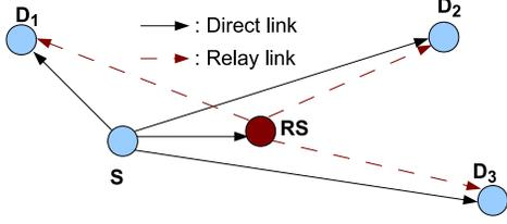
Fig. 1. Two-hop wireless multicasting: Source S transmits common information to destinations  $D_1$ ,  $D_2$  and  $D_3$ , and one RS may assist the source.
