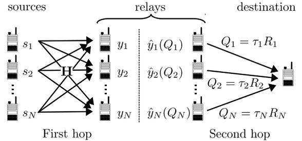
Fig. 1. System setup.
