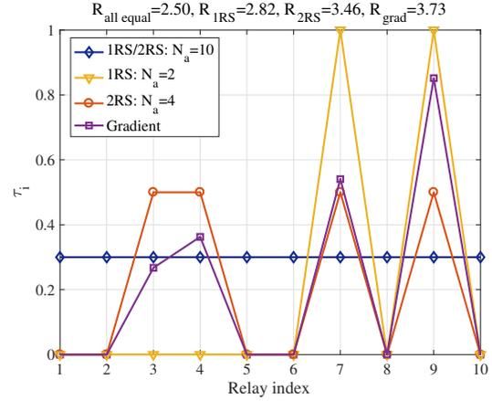
Fig. 6. Instantaneous  $\tau_i$  at the respective peak performance for one specific channel realization in regime III with  $\text{snr} = [2, 4, \dots, 20]$  dB and  $R_i \sim \mathcal{U}(0, 10)$  bps/Hz.
