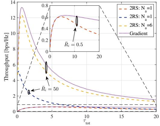
Fig. 8. Total average throughput  $R_{\text{MS}}$  for  $\text{snr} = [2, 4, \dots, 20]$  dB and  $R_i \sim \mathcal{U}(0, 1)$  with average rate  $\bar{R}_i = 0.5$  bps/Hz, and  $R_i \sim \mathcal{U}(0, 100)$  with average rate  $\bar{R}_i = 50$  bps/Hz.
