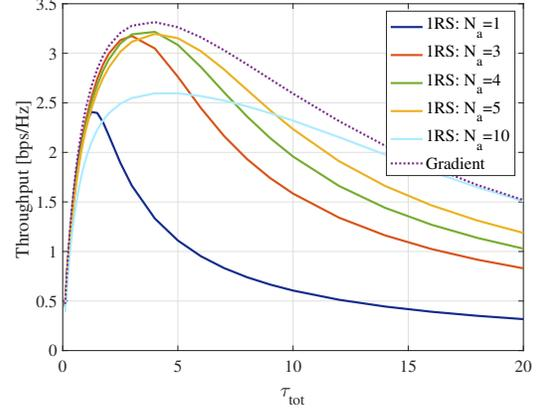
Fig. 4. Total average throughput  $R_{\text{MS}}$  in regime II with  $\text{snr} = [2, 4, \dots, 20]$  dB and  $R_i \sim \mathcal{U}(4.5, 5.5)$  bps/Hz for the first hop relay selection scheme.
