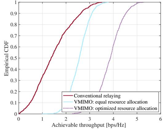
Fig. 2. Achievable throughput of a conventional approach (one relay only), of virtual MIMO with equal resources for all relays and of virtual MIMO with optimized resource allocation.
