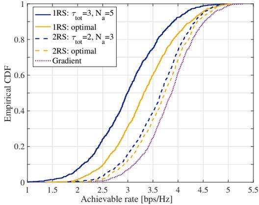
Fig. 7. Instantaneous total throughput at the instantaneous optimal  $\tau_{\text{tot}}$  and  $N_a$ , and at the average optimal  $\tau_{\text{tot}}$  and  $N_a$  in regime III with  $\text{snr} = [2, 4, \dots, 20]$  dB and  $R_i \sim \mathcal{U}(0, 10)$  bps/Hz.
