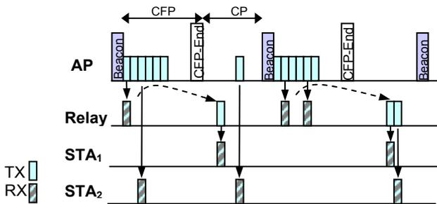
Fig. 1: The first proposed MAC Scheme for relaying
