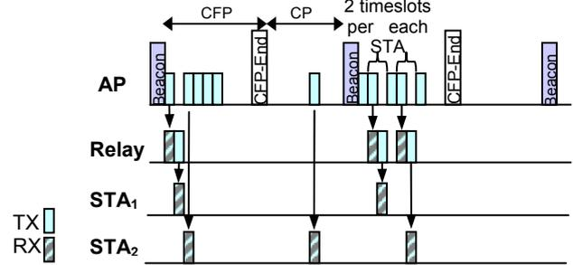
Fig. 2: The second proposed MAC scheme for relaying
