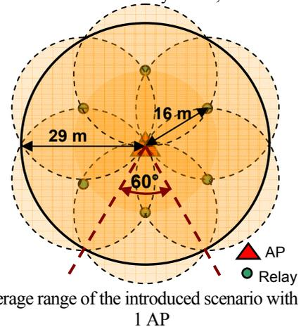
Fig. 5: Coverage range of the introduced scenario with 6 relays and 1 AP
