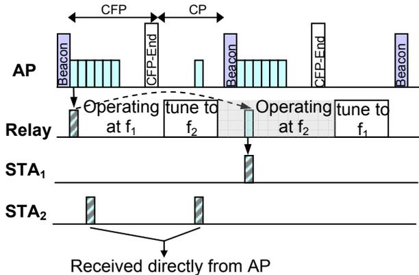
Fig. 3: The third proposed MAC scheme for relaying
