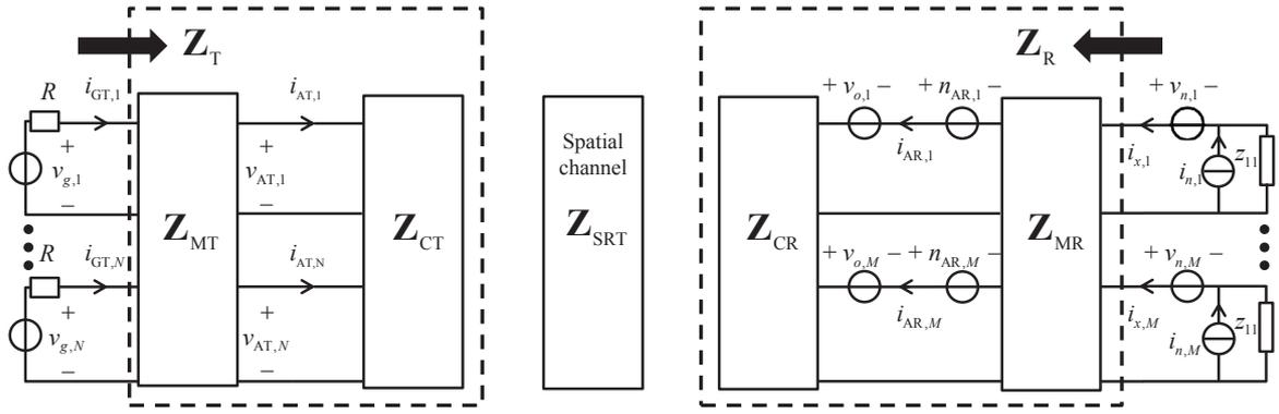
Fig. 1. Circuit model for MIMO communications. The transmitter is on the left and the receiver is on the right.
