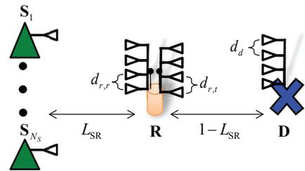
Fig. 2. AF relaying system topology.
