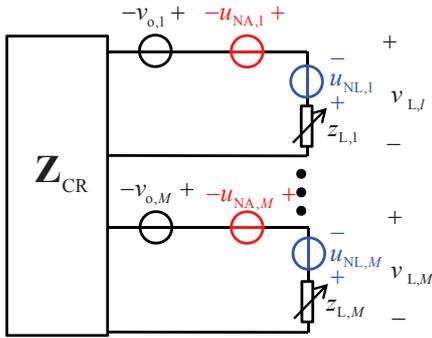
Fig. 1. Circuit model for the receiver of compact MIMO with adaptive load impedances.
