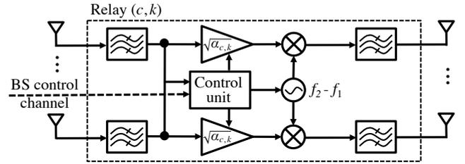
Fig. 1. Conceptual schematic of FDD AF relays.
