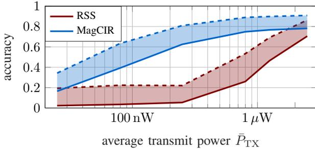
Fig. 8: Accuracy vs. transmit power (solid lines for posture detection, dashed lines for group detection)
