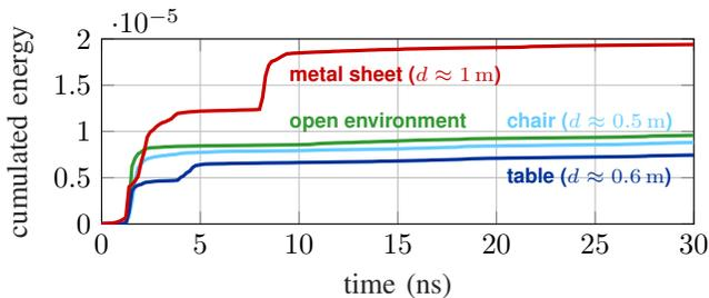
Fig. 4: Cumulated energy of knee-ankle link with different objects in front of the test person
