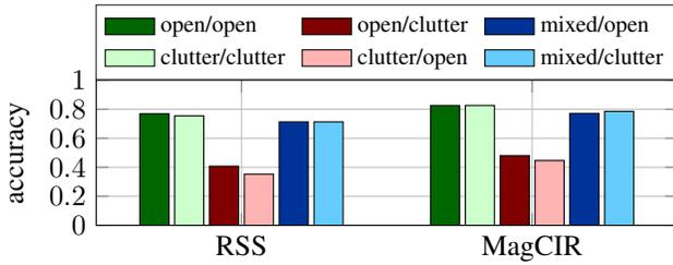
Fig. 7: Accuracy for different training/test data combinations
