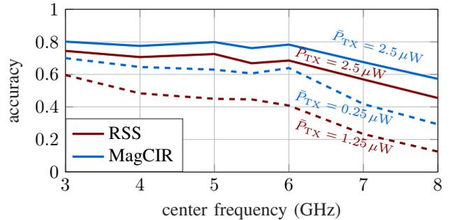
Fig. 6: Accuracy vs. center frequency for different average transmit power levels  $\bar{P}_{TX}$  (w.r.t.  $B = 1$  GHz)
