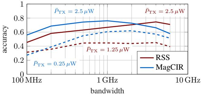
Fig. 5: Accuracy vs. bandwidth for different average transmit power levels  $\bar{P}_{TX}$  (w.r.t.  $B = 1$  GHz)
