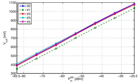
Fig. 5. I/O characteristic of all sMILE nodes, measured with an unmodulated carrier at the input.
