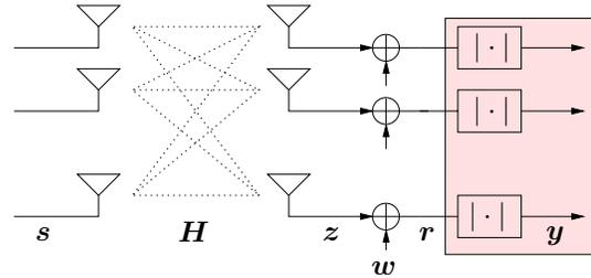
Fig. 1. MIMO Envelope Detection System Model.
