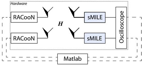
Fig. 2. sMILE testbed hardware block diagram (here for a  $2 \times 2$  MIMO system). Dashed lines correspond to software ‘connections’.
