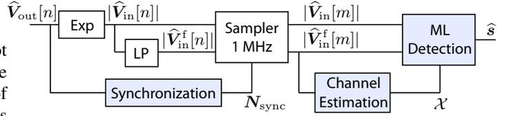
Fig. 6. Block diagram of ‘Processing/Detector’ cell. Corresponds to MIMO processing of the received signals from all sMILE nodes.
