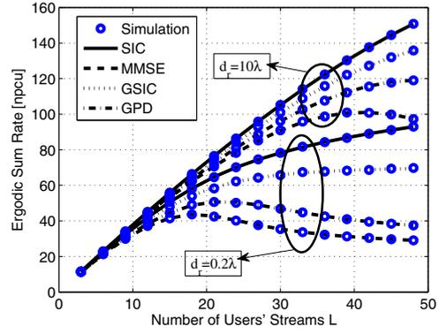
Fig. 1. Sum rate performance of GSIC and GPD for  $\sigma_n^2 = 0$  dB,  $M = 48$  with antenna separation distance  $d_r = 0.2\lambda, 0.5\lambda, L = 3, 6, \dots, 48$  uncorrelated streams and  $t_1 = t_2 = t_3 = L/3$
