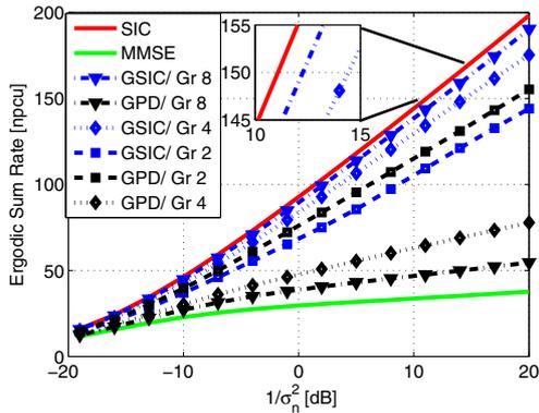
Fig. 2. Rate against  $1/\sigma_n^2$  for using  $\tilde{\Gamma}_{E,\max}$  at  $d_t = 0.2\lambda$ ,  $L = M = 48$ ,  $q = 2, 4, 8$  with  $t_i = L/q\sqrt{i} = 1, \dots, q$ . (best grouping)
