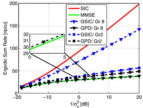
Fig. 4. Rate against  $1/\sigma_n^2$  for using  $\tilde{\Gamma}_{E,\min}$  at  $d_t = 0.2\lambda$ ,  $L = M = 48$ ,  $q = 2, 8$  with  $t_i = L/q\sqrt{i} = 1, \dots, q$ . (worst grouping)
