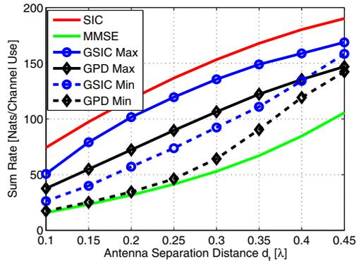
Fig. 5. Maximum and minimum rates for GSIC and GPD Vs.  $d_t$  for  $L = M = 48$  at  $\sigma_n^2 = -5\text{dB}$ ,  $q = 3$  and  $t_1 = t_2 = t_3 = 16$ .
