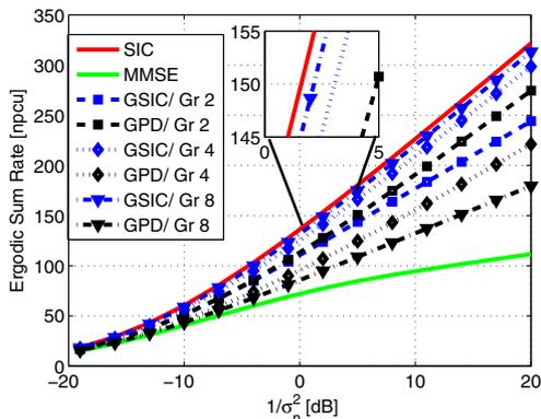
Fig. 3. Rate against  $1/\sigma_n^2$  for using  $\tilde{\Gamma}_{S,\max}$  at  $d_t = 0.4\lambda$ ,  $L = M = 48$ ,  $q = 2, 4, 8$  with  $t_i = L/q\sqrt{i} = 1, \dots, q$ . (best grouping)
