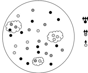
Fig. 1. Heterogeneous wireless ad hoc network. A cloud indicates an underlying wireless personal area network.
