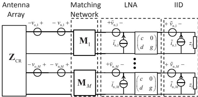
Fig. 1: Circuit model for the receiver of compact MIMO.
