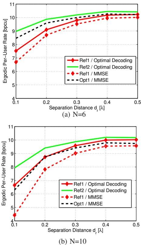
Fig. 3: Average per-user rate versus the antenna separation distance for  $N = 6$  and  $N = 10$  users at  $\text{SNR} = 15$  dB.
