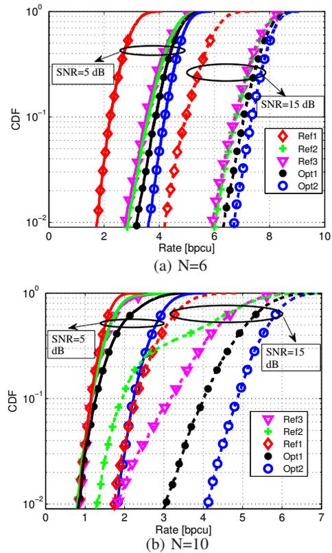
Fig. 4: Minimum rate given an MMSE equalizer for  $N = 6, 10$ ,  $M = 30$ ,  $d_r = 0.1\lambda$  and SNR = 5, 15dB.
