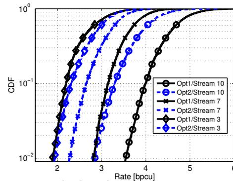
Fig. 5: CDF of (3<sup>rd</sup>, 7<sup>th</sup>, 10<sup>th</sup>) sorted rates for MMSE equalizer,  $N = 10$ ,  $M = 30$ ,  $d_r = 0.1\lambda$  and SNR = 5dB.
