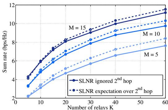
Fig. 5. Achievable sum rates for different network configurations with relays.
