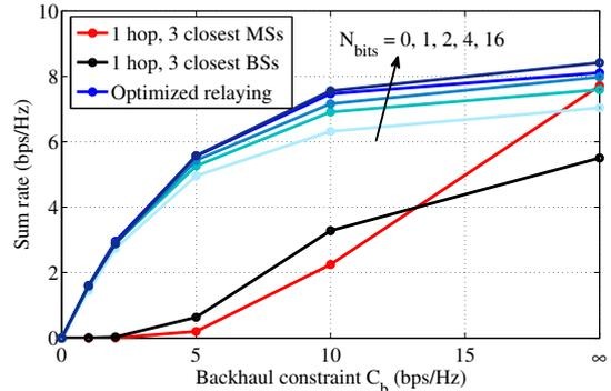
Fig. 6. Influence of power control for different BS backhaul constraints.
