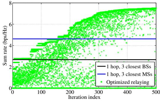
Fig. 4. Convergence behavior of the sum rate maximization for a typical network realization with relays.
