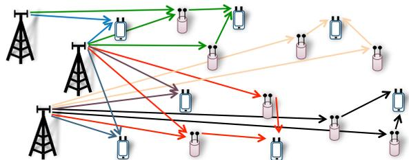
Fig. 1. A “post-cellular” network in which a cluster of BSs serves a wide area by the assistance of many distributed low-complexity relays.
