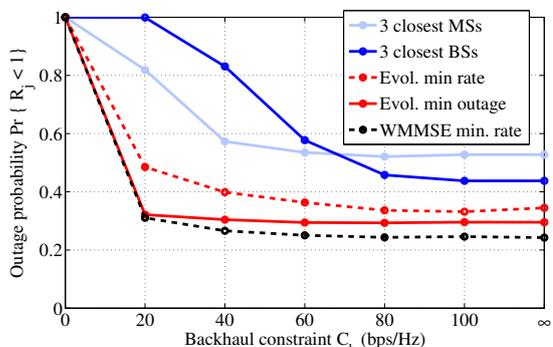
Fig. 3. The probability that a mobile user is in outage for different backhaul rate constraints.
