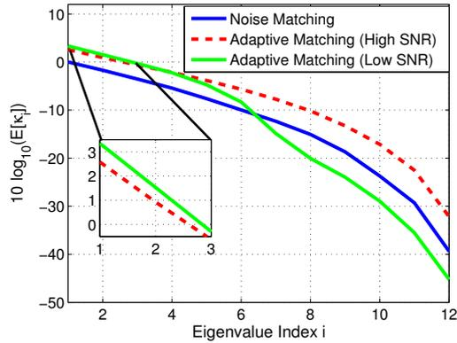
Fig. 5: Average eigenvalues for  $N = 12$  users and  $M = 30$  antennas for very high SNR and very low SNR.
