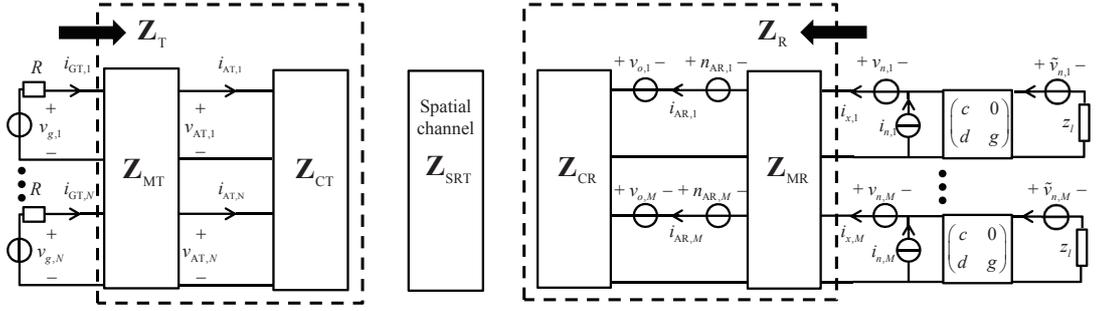
Fig. 1: Circuit model for MIMO communications. The transmitter is on the left and the receiver is on the right.
