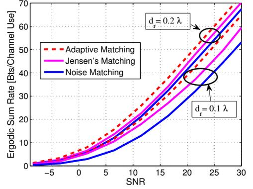
Fig. 4: Rate scaling against SNR for  $N = 8$  users, and  $M = 30$  antennas at the receiver for antenna spacings of  $d_r = 0.1\lambda$  and  $d_r = 0.2\lambda$ .
