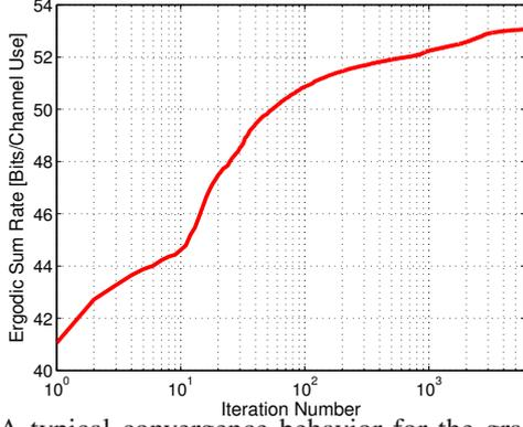
Fig. 2: A typical convergence behavior for the gradient algorithm for  $N = 12$  and  $M = 30$  antennas at SNR=12dB.
