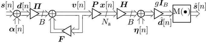
Fig. 5. Scaled Vector Precoding Reference Model.
