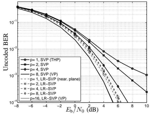
Fig. 8.  $B = N_a = 8$ , Zero-Forcing Variant, SVP and LR-SVP
