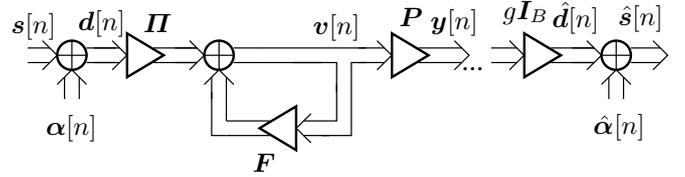
Fig. 3. Equivalent Linear Representation without the Modulo Operators.
