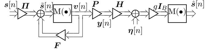
Fig. 2. Block Diagram for Tomlinson-Harashima Precoding.
