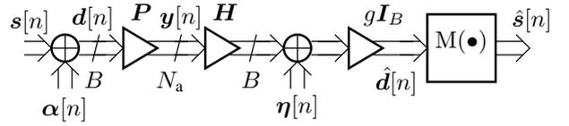
Fig. 4. Vector Precoder System Model.
