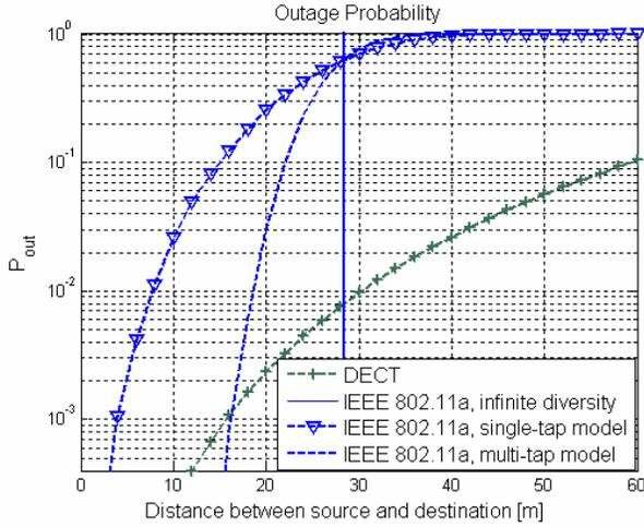
Fig. 1. Outage probability for a system based on IEEE 802.11a and DECT.
