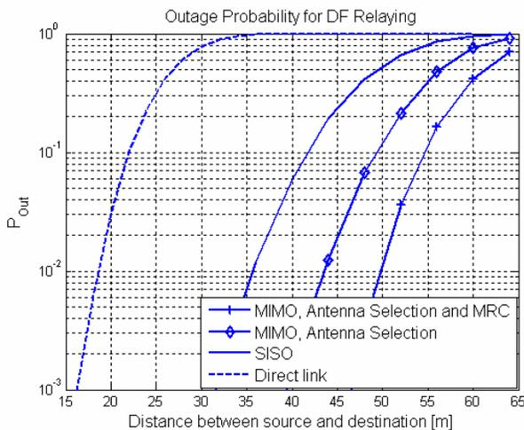
Fig. 5 Outage Probability for DF in MIMO case with two antennas per each node
