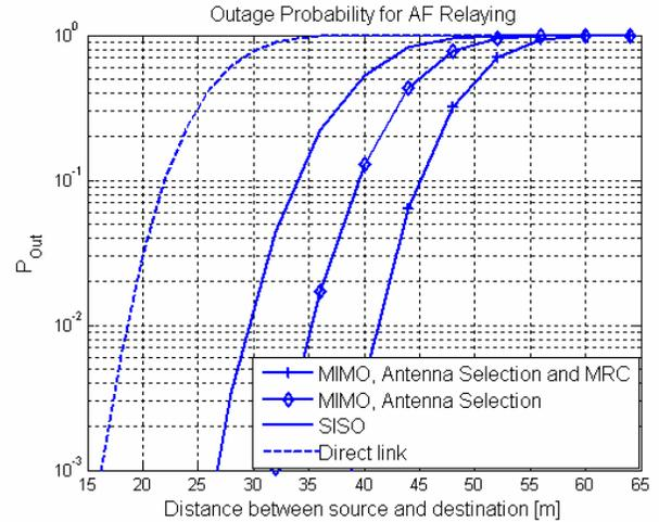
Fig. 6 Outage Probability for AF in MIMO case with two antennas per each node
