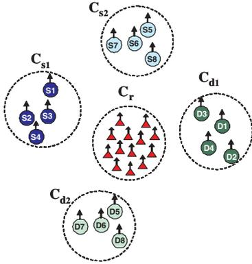
Fig. 1. A MUZFR network with 13 AF relays, 8 sources and 8 destinations. Each source- and destination-cluster consists of 4 STAs.
