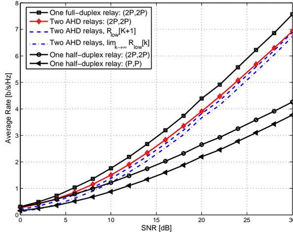
Figure 1: Average rates vs. signal-to-noise ratio for  $\nu_1^2 = 1$ ,  $\nu_2^2 = 1$ ,  $\nu_{12}^2 = 0.5$ ,  $K = 50$  and full interference cancellation
