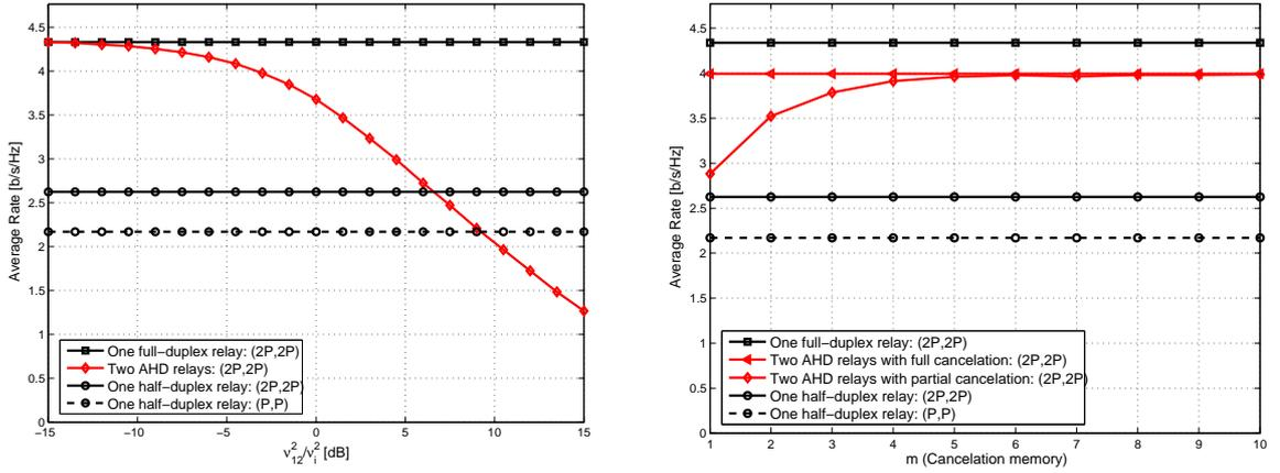
(a) Average rate vs. relative strength of the inter-relay channel (with respect to source-relays and relays-destination channel variances  $\nu_1^2 = \nu_2^2 = 1$ ) for SNR=20dB
