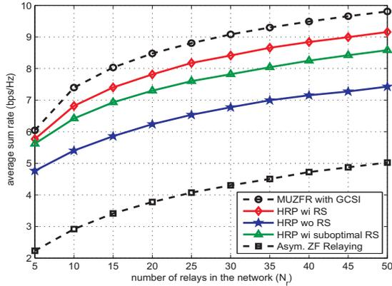
Fig. 2. Average sum rates vs.  $N_r$  for  $N = 2$ ,  $N_{r,2} = 2$  (i.e., minimum relay configuration for  $C_{\text{global}}$ ), SNR = 20 dB.
