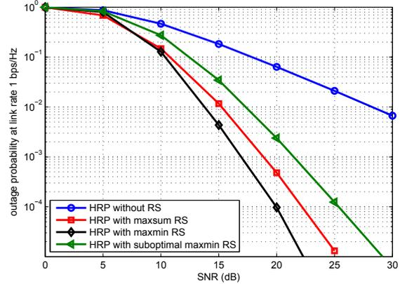
Fig. 3. The outage probability vs. SNR for  $N = 2$ ,  $N_r = 6$ ,  $N_{r,2} = 2$  (i.e., minimum relay configuration for  $C_{\text{global}}$ ).
