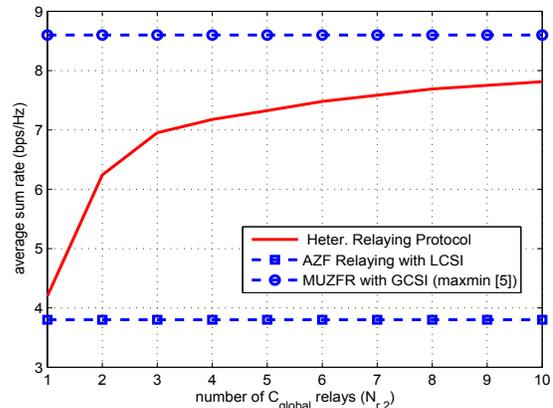
Fig. 4. Average sum rates vs.  $N_{r,2}$  for the excess relays case in  $C_{\text{global}}$  and  $N = 2$ ,  $N_r = 20$ , SNR = 20 dB.
