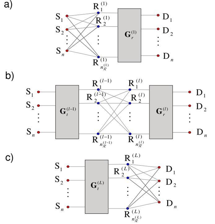
Fig. 2. Receive (a), joint transmit/receive (b), transmit (c) beamforming.
