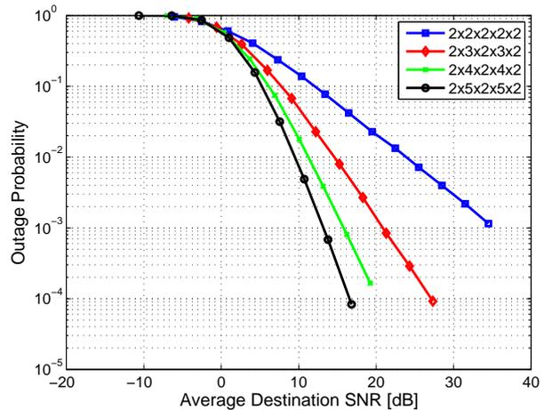
Fig. 4. Outage probability versus SNR for various four-hop networks. The code rate is fixed to  $R = 1$  bit/channel use which corresponds to  $r = 0$ .
