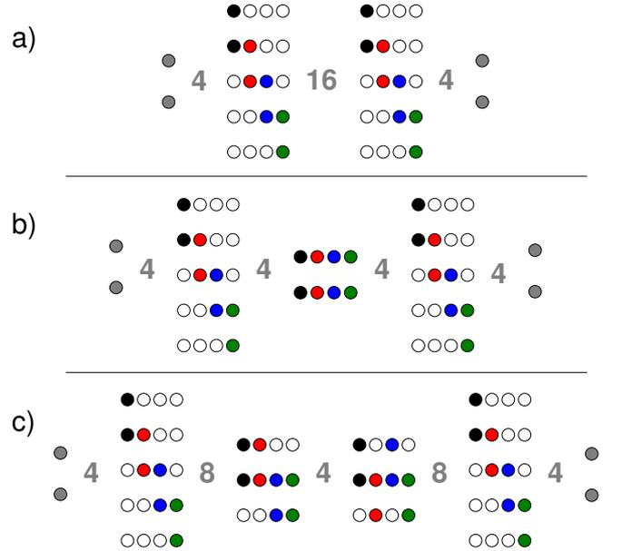
Fig. 3. Relay set selection algorithm applied to different topologies with  $\bar{d}(0) = 4$ :  $2 \times 5 \times 5 \times 2$  (a),  $2 \times 5 \times 2 \times 5 \times 2$  (b),  $2 \times 5 \times 3 \times 3 \times 5 \times 2$  (c). Selected relays: black (cycle 1), red (cycle 2), blue (cycle 3), green (cycle 4). Bounds  $\bar{d}_i(0)$  are indicated in grey.
