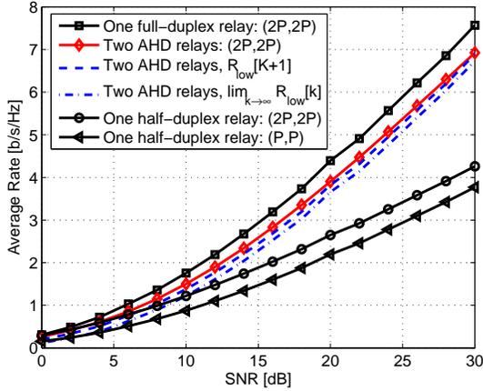
Fig. 2. Two-path relaying with amplify-and-forward and  $\nu_{12}^2 = 0.5$
