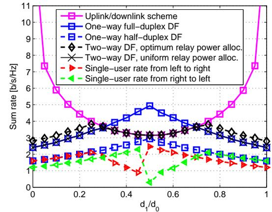
Fig. 5. Sum rate for two-way relaying with decode-and-forward
