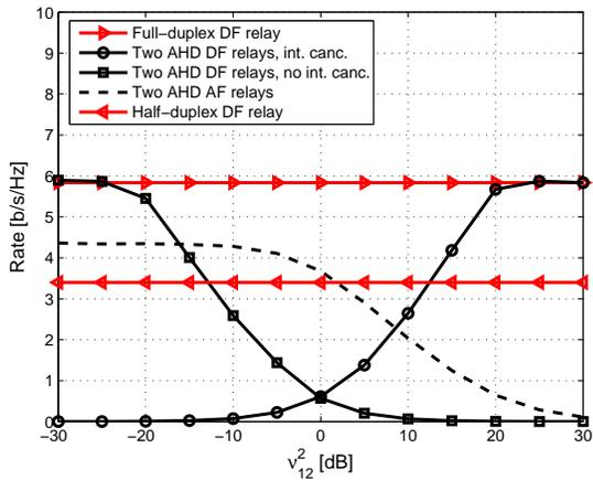
Fig. 3. Two-path relaying with decode-and-forward and SNR=20dB
