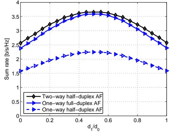
Fig. 4. Sum rate for two-way relaying with amplify-and-forward
