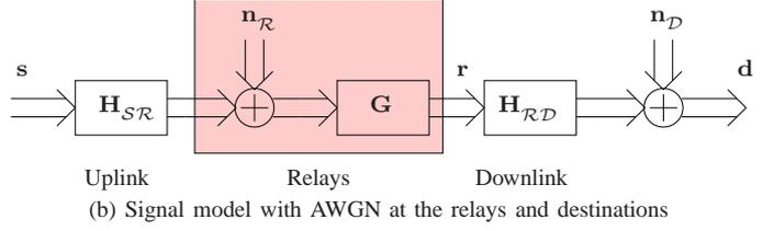
Fig. 1. System configuration and compound signal model for a two-hop relay network
