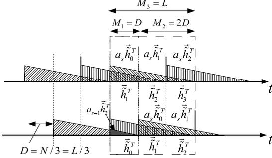
Fig. 4. Signal example of non-delayed and delayed correlation input in presence of moderate ISI with  $N = L$  and  $D = N/3$ .
