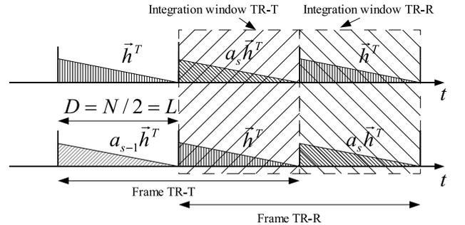
Fig. 2. Signal example of non-delayed and delayed correlation input in absence of ISI with  $N/2 = L$ .
