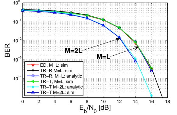
Fig. 5. BER of transmitted reference in absence of ISI with  $D = N/2 = L$
