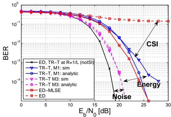
Fig. 6. BER of transmitted reference in case of moderate ISI with  $D = N/3 = L/3$ .
