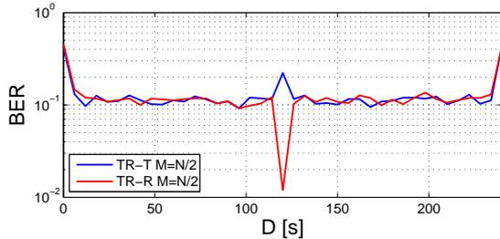
Fig. 7. BER of TR-T and TR-R in case of moderate ISI and fixed integration duration  $M = N/2 = L/2$  as a function of delay  $D$ .
