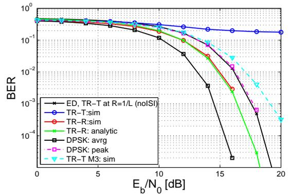
Fig. 8. BER performance for TR-T and TR-R with  $D = N/2 = L/2$  and DPSK
