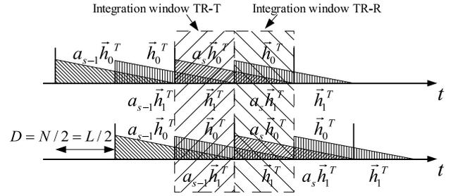
Fig. 3. Signal example of non-delayed and delayed correlation input in presence of moderate ISI with  $N = L$  and  $D = N/2$ .
