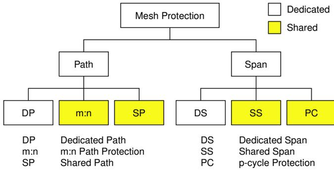
Fig. 2. Different protection schemes in mesh networks.
