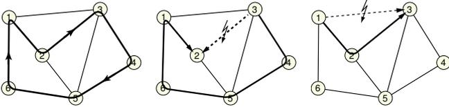
Fig. 3.  $p$ -cycle protection. From left to right: network with established  $p$ -cycle, failure of an on-cycle and of a straddling span.
