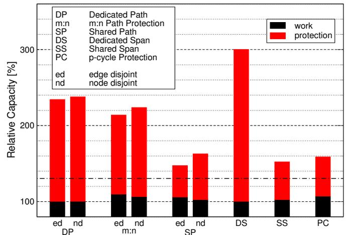
Fig. 7. Capacity requirements for the TT network of the COST 266 action.
