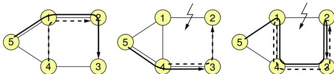
Fig. 1. Differences between path and span protection (from left to right: working state, path protection, and span protection).
