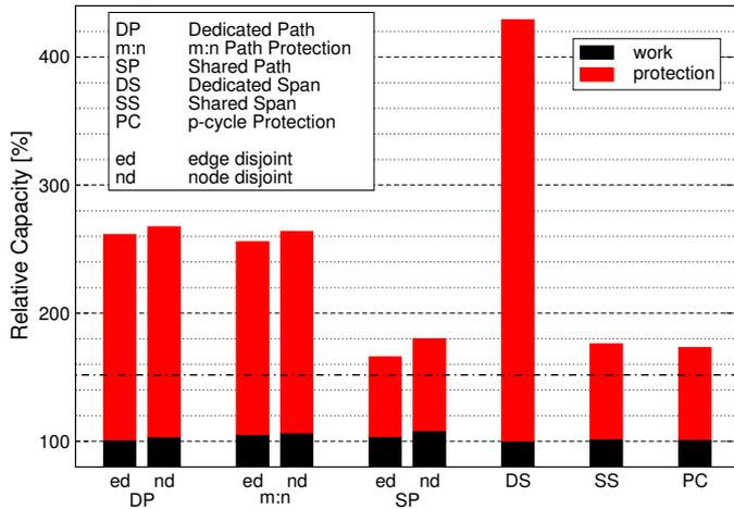
Fig. 5. Capacity requirements for the BT network of the COST 266 action.
