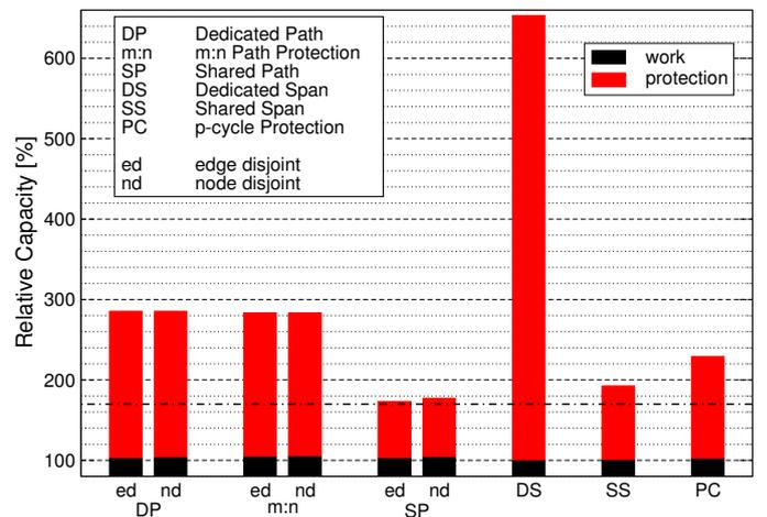
Fig. 6. Capacity requirements for the RT network of the COST 266 action.
