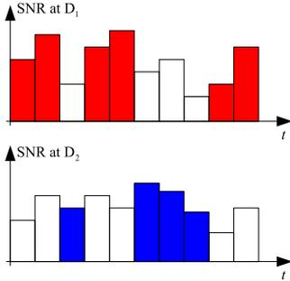
Fig. 6. Adaptive scheduling depending on the SNR at the destinations
