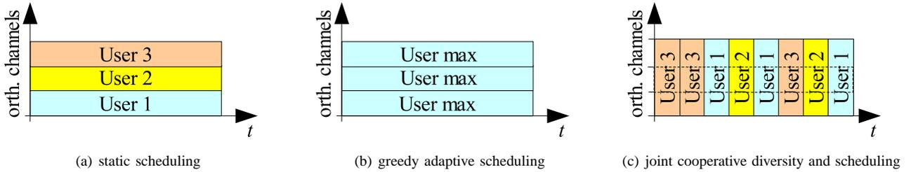
Fig. 5. Use of orthogonal channels in the network in different scheduling scenarios
