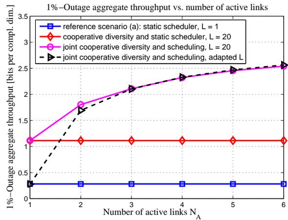
Fig. 9. 1%-Outage aggregate throughput;  $P/\sigma^2 = 20\text{dB}$  and  $\sigma^2 = \sigma_R^2$
