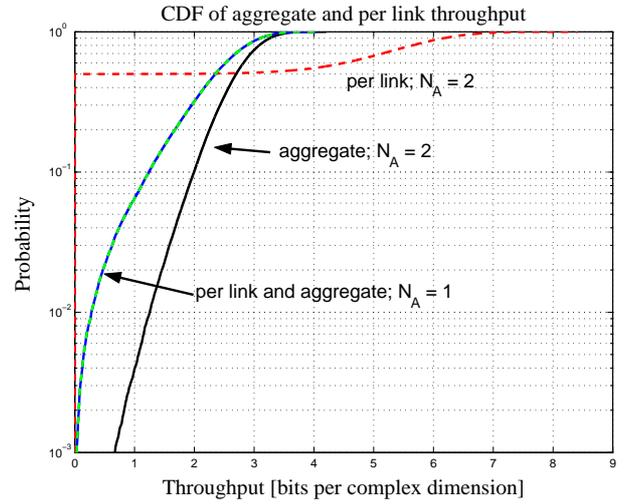
Fig. 4. CDF of the aggregate (solid lines) and the per-link throughput (dashed lines) for the static fading environment;  $P/\sigma^2 = 20\text{dB}$ ,  $\sigma^2 = \sigma_R^2$ , and  $L = 1$ .
