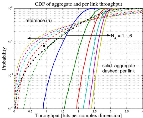
Fig. 8. CDF of the aggregate (solid lines) and the per link throughput (dashed lines) for the joint cooperative diversity and scheduling scenario;  $P/\sigma^2 = 20\text{dB}$  and  $\sigma^2 = \sigma_R^2$
