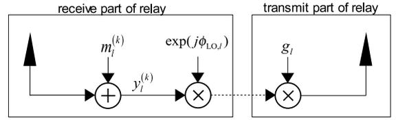
Fig. 2. System model of amplify-and-forward relay
