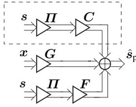
Fig. 2. Equivalent model without the quantizer for SDFE and DFE, with and without the dashed box, respectively.
