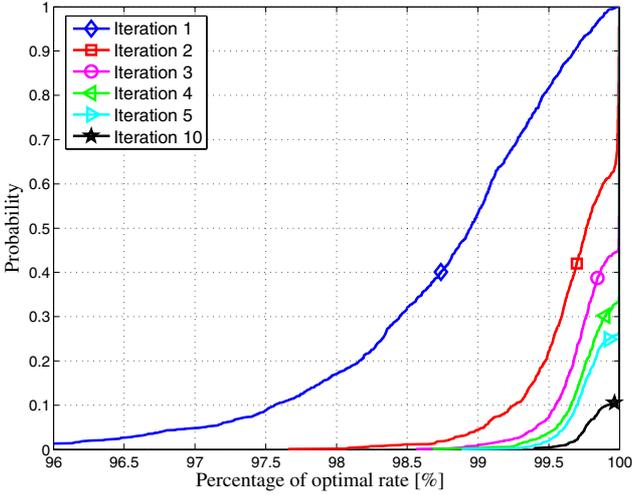
Fig. 1. CDFs of percentage of optimal rate obtained by iterative optimization for different number of iterations; equal transmit power, i.e.,  $P_S = P_R$ ; uniform power delay profile;  $L = 4$ ;  $N_{\text{fft}} = 16$ ;  $\rho_0 = 0\text{dB}$ ;  $d_r = d_1/d_0 = 0.5$
