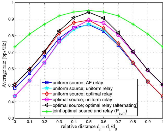
Fig. 3. Normalized average rate vs. relative distance with pairing of subcarrier and equal transmit power, i.e.,  $P_S = P_R$ ; uniform power delay profile;  $L = 4$ ;  $N_{fft} = 16$ ;  $\rho_0 = 0\text{dB}$ ;
