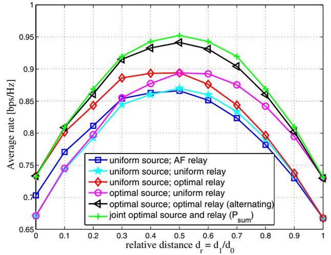
Fig. 4. Normalized average rate vs. relative distance with pairing of subcarrier and joint average transmit power according to (13) and (14); uniform power delay profile;  $L = 4$ ;  $N_{fft} = 16$ ;  $\rho_0 = 0\text{dB}$ ;
