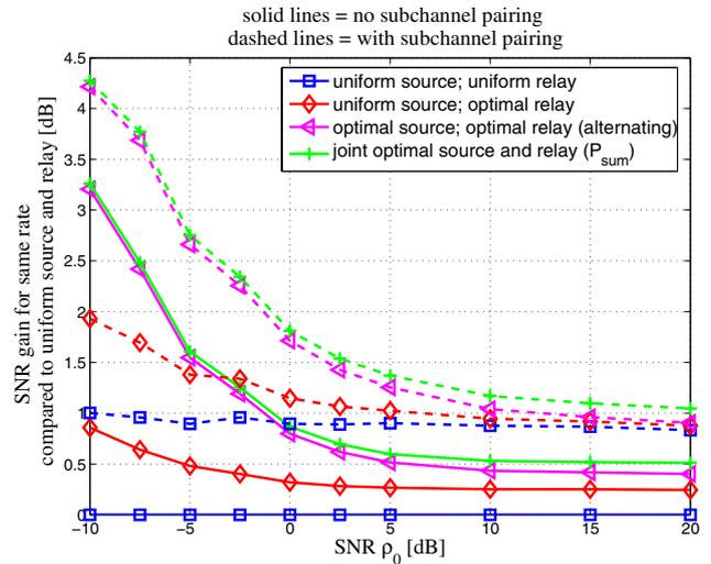
Fig. 5. SNR gain [dB] to achieve same average rate as uniform PA at source and relay without pairing of subchannels; uniform power delay profile;  $L = 4$ ;  $N_{fft} = 16$ ;  $d_r = 0.5$
