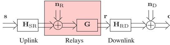
Fig. 2. Block diagram with AWGN at the relays and destinations
