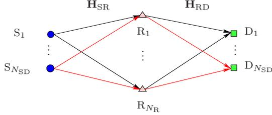
Fig. 1. Two hop system configuration with half-duplex relays
