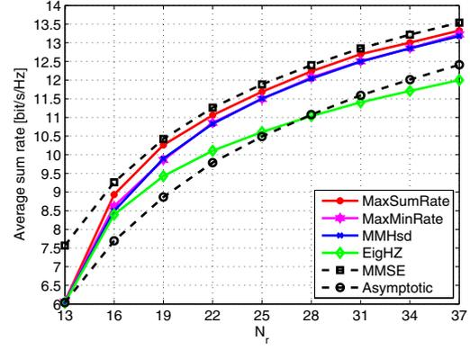
Fig. 4. Average sum rate vs.  $N_R$  for  $N_{SD} = 4$  and  $\text{SNR}_{\text{def}} = 10$  dB.
