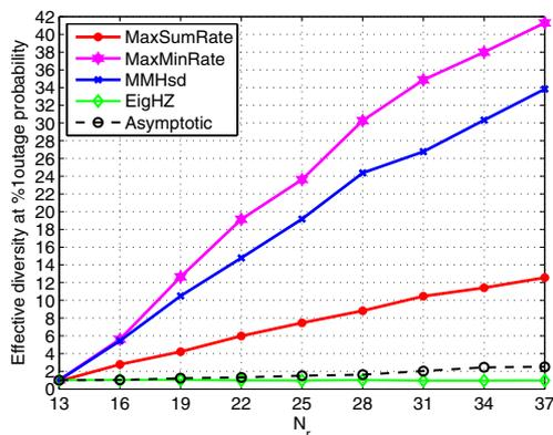
Fig. 6. Effective diversity at %1 outage probability vs.  $N_R$  for  $N_{SD} = 4$  and  $SNR_{def} = 10$  dB.
