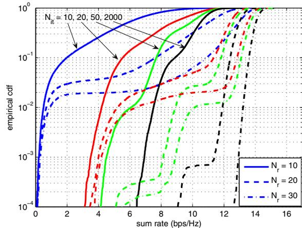
Figure 4. Three source-destination pairs: Empirical CDFs of the achievable sum-rate for various numbers of relays  $N_r$  and outer iterations  $N_{it}$  in the gradient algorithm (SNR = 25 dB).
