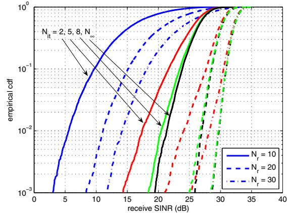
Figure 2. Single source-destination pair in the presence of two interference sources: Empirical CDFs of receive SINR for different numbers of relays  $N_r$  and outer iterations  $N_{\text{it}}$  in the gradient algorithm (SNR = 25 dB).
