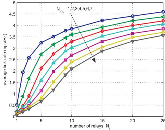
Figure 1. Single source-destination pair in the presence of  $N_{\text{int}}$  interference sources: Average achievable link rates versus number of relays  $N_r$  with optimal relay gain allocation (SNR = 20 dB).
