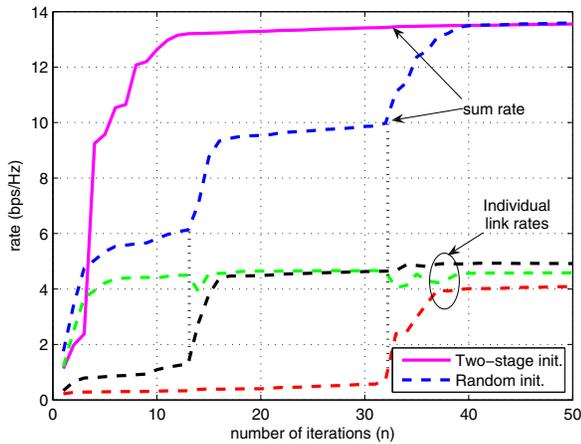
Figure 3. Three source-destination pairs: Sample trajectory of achievable rates at each outer iteration for a typical channel realization with  $N_r = 30$ .
