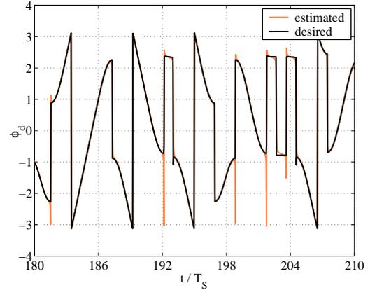
Fig. 9. Subspace phase estimate, 1 -  $D$ -channel
