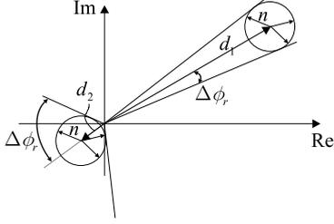
Fig. 5. Phase error for high and low amplitude
