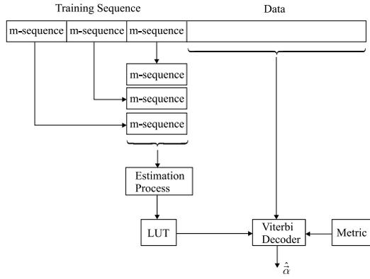
Fig. 3. Decoding of a data burst
