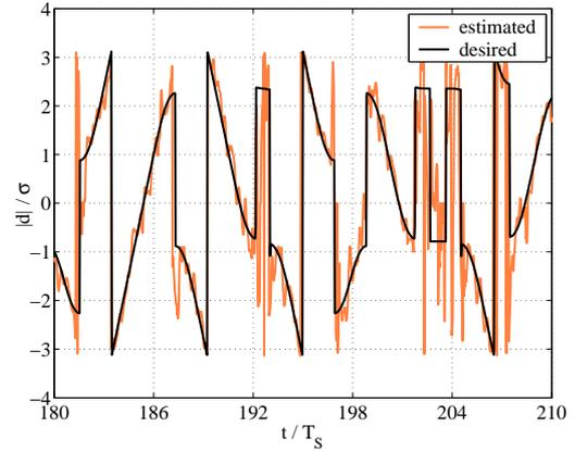
Fig. 4. First phase estimate, 1 -  $D$ -channel
