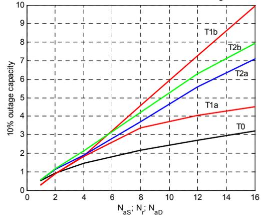
Fig. 4: 10% outage capacity versus the number of source/destination antenna elements.
