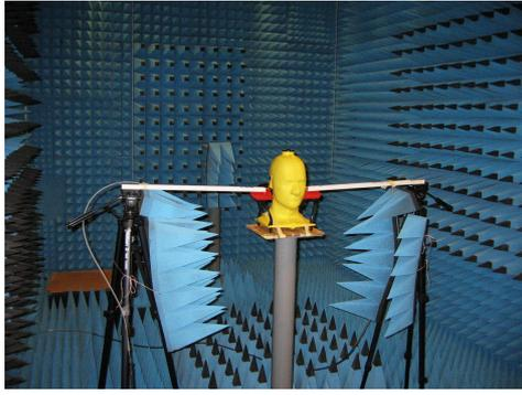
Fig. 1. Measurement setup with head phantom in the anechoic chamber
