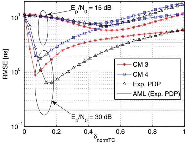
Fig. 4. RMSE for TC (3) as function of  $\delta_{\text{normTC}}$  for all channel models.
