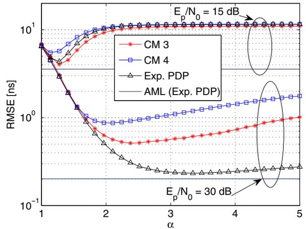
Fig. 2. RMSE for IWI (6) as function of  $\alpha$  for all channel models.
