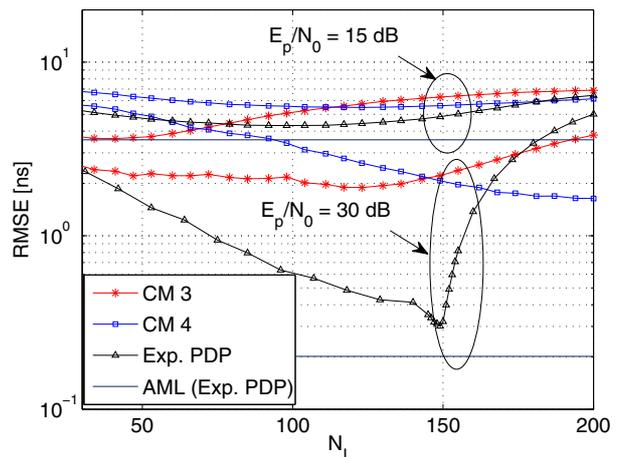
Fig. 3. RMSE for SW (4) as function of  $N_I$  for all channel models.
