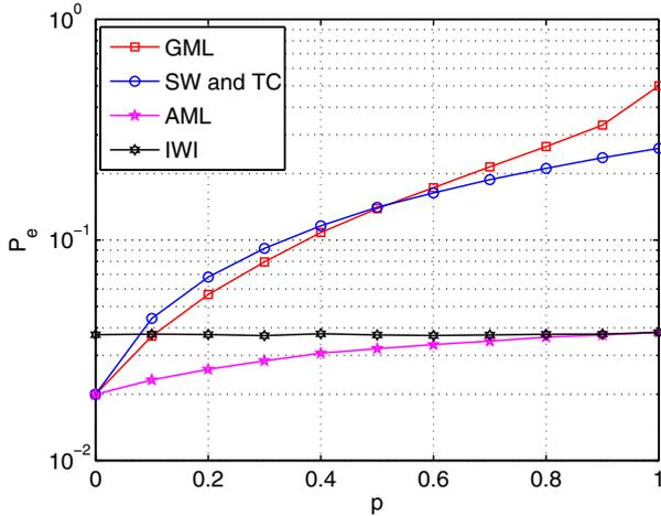
Fig. 1.  $P_e$  for GML (10), SW and TC (8), AML (7), IWI (9) as function of  $p$  and  $\text{SNR}_{\text{toy}} = 30$  dB.
