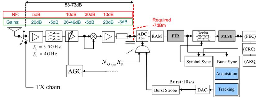
Fig. 1. Block diagram of UWB-IR receiver with MLSE post-detection
