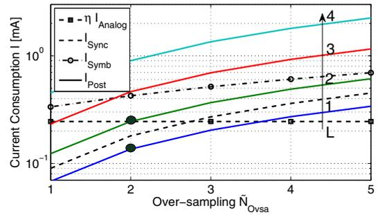
Fig. 4. Analog and digital receiver currents.
