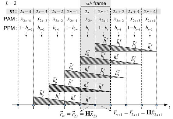
Fig. 2. Schematic construction of noiseless receive signal in the  $s$ th frame (half-slots:  $2s$  and  $2s + 1$ ) in case of  $L = 2$
