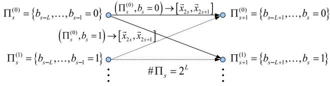
Fig. 3. Generic structure of the Viterbi decoder
