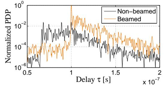
Fig. 8. Instantaneous PDP example of a beamed and a non-beamed receive signal
