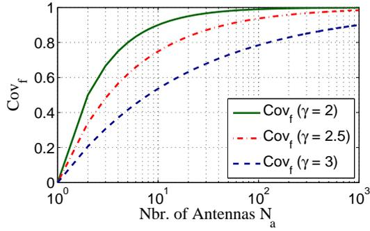
Fig. 4. Feasibility coverage as a function of  $N_a$  for different path loss exponents  $\gamma$
