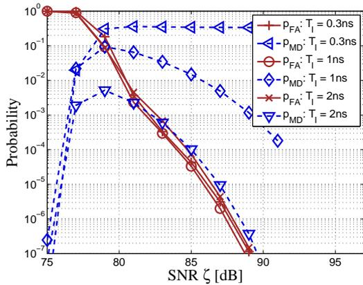
Fig. 10. Probabilities  $p_{FA}$  and  $p_{MD}$  for  $R_D = 100$  m,  $N_a = 10$ ,  $\gamma = 2$ ,  $\tilde{\eta} = 0.7$ , and different bandwidth  $B = 1/T_1$ , if jitter of 1 ns is present
