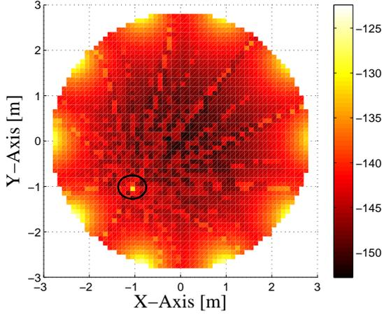
Fig. 6. Beam pattern  $y_{\max}(i, j)$  [dB] over disc, if beamforming is done to position  $(x_0, y_0) = (-1, -1)$  m; for  $N_a = 10$ ,  $B = 3$  GHz, and  $\gamma = 2$ .
