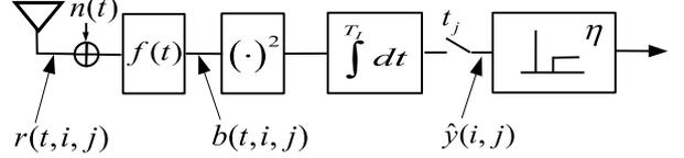
Fig. 3. Signal model of the wake-up detector
