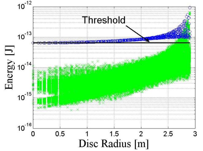
Fig. 7. All beamed samples, i.e.,  $y_{\max}(i, i)$ ,  $\forall i$  (o) and all non-beamed samples, i.e.,  $y_{\max}(i, j)$ ,  $\forall i$  and  $\forall j \setminus i$  (x) plotted over disc radius; for  $N_a = 10$ ,  $B = 3$  GHz, and  $\gamma = 2$ .
