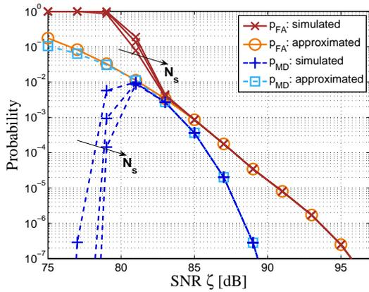
Fig. 9. Probabilities  $p_{FA}$  and  $p_{MD}$  for  $R_D = 100$  m,  $N_a = 10$ ,  $B = 3$  GHz,  $\gamma = 2$ ,  $\tilde{\eta} = 0.5$ , and different  $N_s$ .
