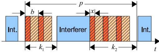
Fig. 2. Scheme to determine the maximum pulse rate with interfering bursts (solid) and UWB packets (lined)
