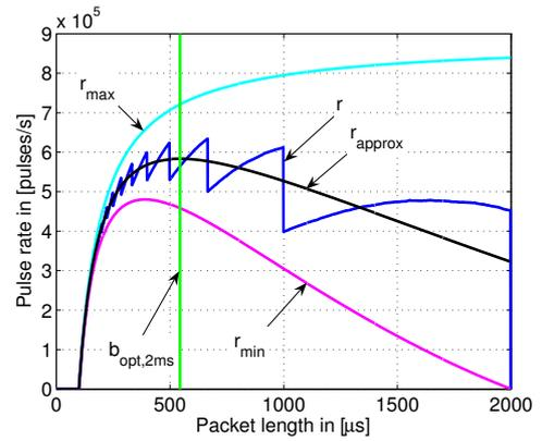
Fig. 6. Achievable UWB pulse rate with one GSM interferer present, assuming  $p = 2\text{ms}$  and  $x = 100\mu\text{s}$
