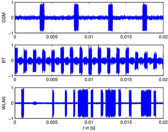
Fig. 1. Measured time domain signals of GSM, BT, and WLAN
