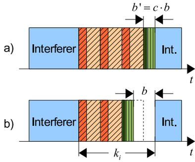
Fig. 3. UWB packet distribution in an unoccupied slot of duration  $k_i$ , a) using  $r_{\max}(b)$  from (3), and b) using  $r_{\min}(b)$  from (4); Interferer bursts are plotted solid, UWB packets are plotted diagonal lined, and fractional UWB packets are vertical lined
