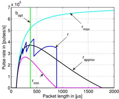
Fig. 9. Achievable UWB pulse rate with one BT interferer present, assuming  $p = 2\text{ms}$  and  $x = 100\mu\text{s}$
