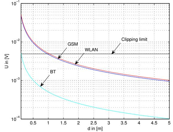
Fig. 5. Signal amplitudes of interferers at the UWB receiver considering free space attenuation and a 5th order Butterworth filter with  $f_l = 3.1\text{GHz}$
