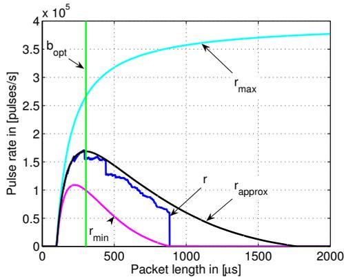
Fig. 13. Achievable UWB pulse rate with three GSM, three 802.11b WLAN, and one BT interferer present at the same time, assuming  $p = 2\text{ms}$  and  $x = 100\mu\text{s}$
