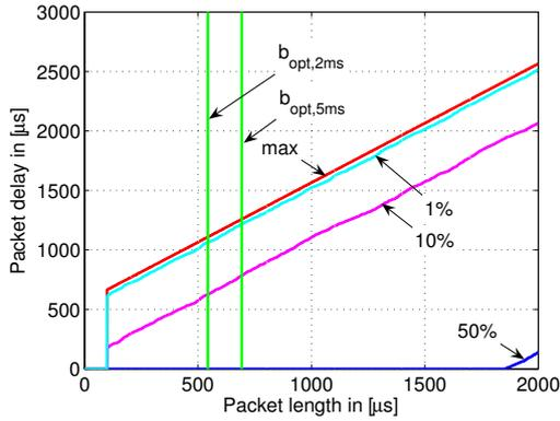
Fig. 8. Packet delays with one GSM interferer present
