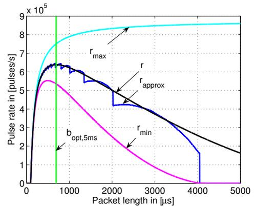
Fig. 7. Achievable UWB pulse rate with one GSM interferer present, assuming  $p = 5\text{ms}$  and  $x = 100\mu\text{s}$
