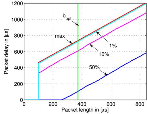
Fig. 10. Packet delays with one BT interferer present
