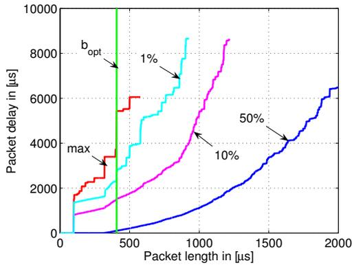
Fig. 12. Packet delays with one WLAN interferer present
