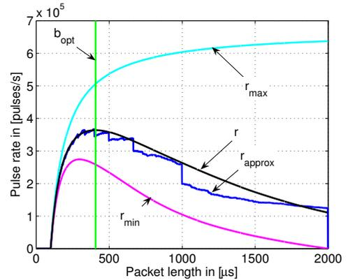
Fig. 11. Achievable UWB pulse rate with one WLAN interferer present, assuming  $p = 2\text{ms}$  and  $x = 100\mu\text{s}$
