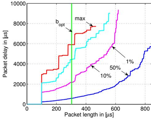
Fig. 14. Packet delays with three GSM, three 802.11b WLAN, and one BT interferer present at the same time
