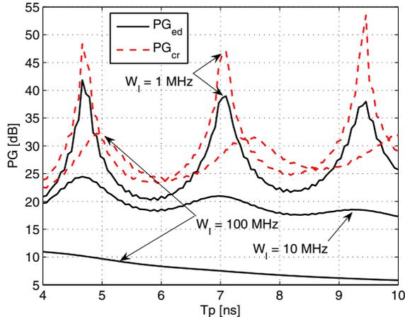
Fig. 7. Processing gains for correlation receiver and energy detection receiver for increasing  $T_p$
