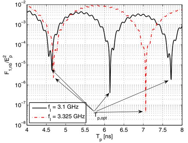
Fig. 3. First part of the variance of  $I_{\text{ed}}$  for fixed  $f_I$  and varying  $T_p$
