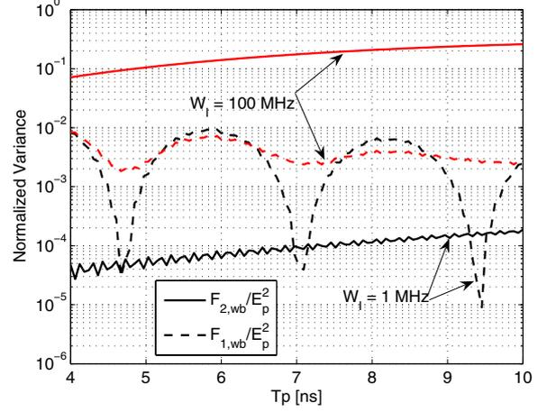
Fig. 5. Variance of  $I_{ed}$  for varying integration times  $T_p$
