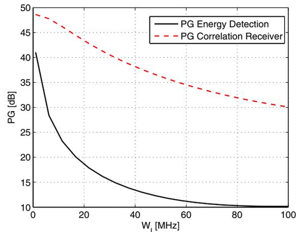
Fig. 8. Processing gains for correlation receiver and energy detection receiver for increasing  $W_I$
