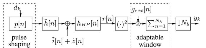
Fig. 1. Discrete time system model.
