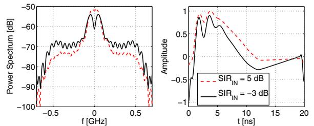
Fig. 4. Optimized window functions in frequency and time domain for  $E_b/N_0 = 14.6$  dB and optimized pulse shapes.
