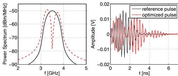
Fig. 2. Reference pulse and optimized pulse in frequency and time domain for  $E_b/N_0 = 24.2$  dB and  $SIR_{IN} = 5$  dB.
