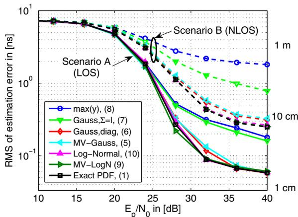
Fig. 4. Performance of Timing Estimators for LOS and NLOS Channel
