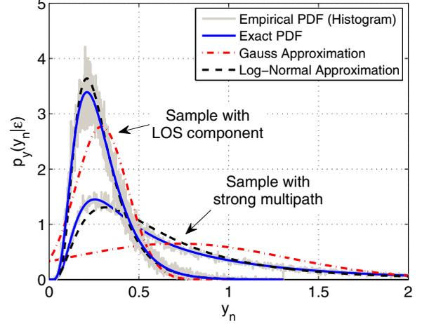
Fig. 2. Exact PDF of ED output sample compared to histogram and closed form approximations
