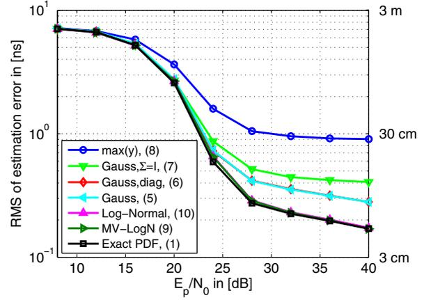
Fig. 3. Performance of timing estimators for normally distributed CIRs with exponential PDP
