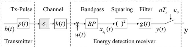
Fig. 1. Block diagram of transmitter, channel and receiver
