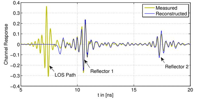
Fig. 2. Reconstructed and measured channel response of controlled anechoic chamber environment with two reflectors
