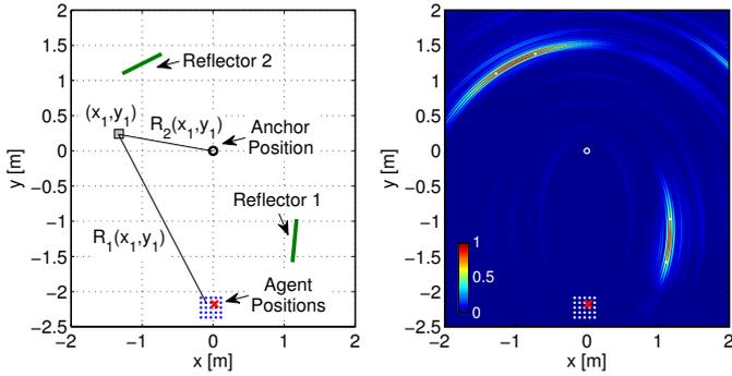
Fig. 1. Anechoic chamber measurements with two reflectors: setup (left) and magnitude of scattering coefficient map (right)
