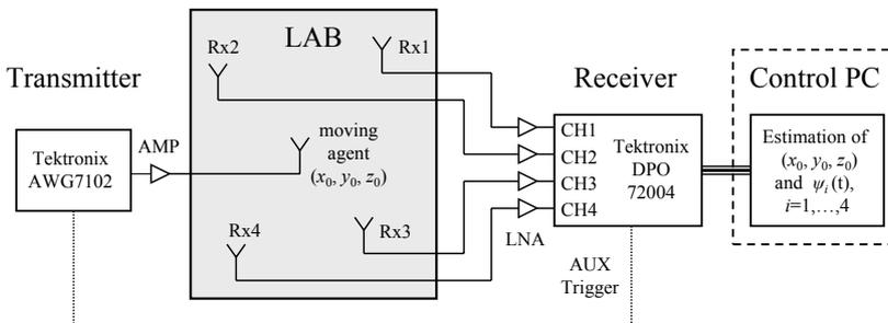
Fig. 3. Schematic diagram of measurement setup and photo of laboratory and measurement equipment
