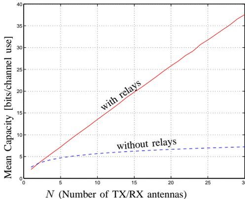
Fig. 2. Mean capacity of a  $N \times N$  MIMO link with and without relay nodes for free space propagation and number of relays  $R = 112$
