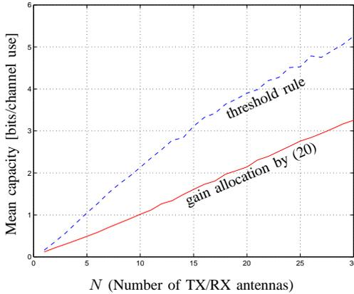
Fig. 7. Comparison of mean capacity for gain allocation with threshold rule and gain allocation by (20) with  $Q_l = 1 \forall l$
