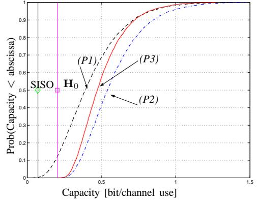
Fig. 5. Cumulative Distribution Functions of the capacity for protocol scenarios (P1)-(P3),  $\{N, M, R, \sigma_r^2, \sigma^2, g_{th}\} = \{3, 3, 80, 10^{-5}, 10^{-5}, 45\text{dB}\}$ , mean values are plotted at the 50% percentile of the CDFs
