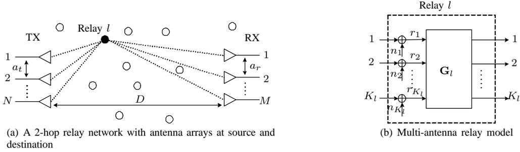
Fig. 1. Relay network with linear relay nodes
