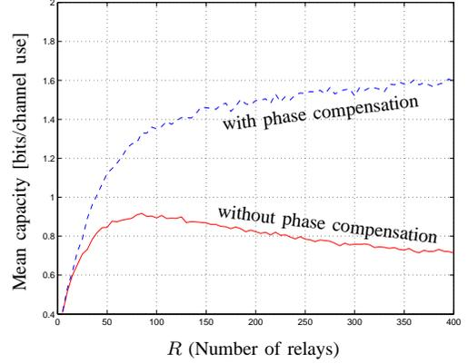
Fig. 8. Mean Capacity with and without phase compensation at the relays and destination with  $N = M = 5$ , gain allocation by (20)
