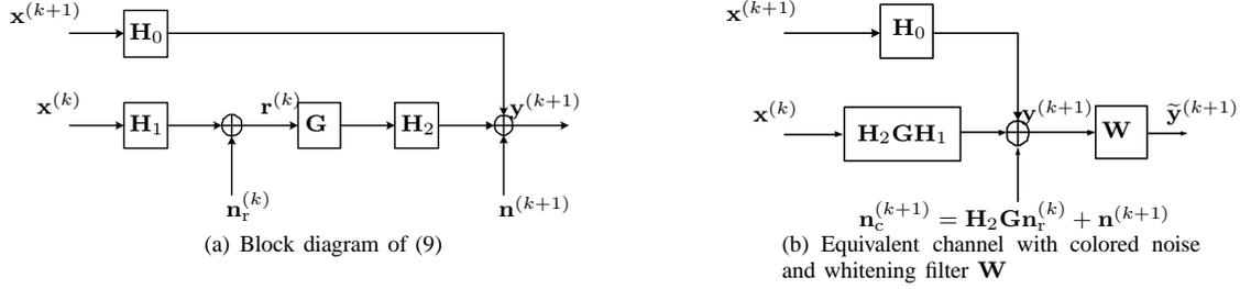
Fig. 3. Block diagrams of received signal at the destination in time slot  $k + 1$
