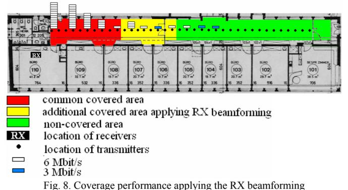
Fig. 8. Coverage performance applying the RX beamforming
